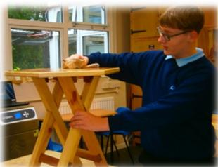
**Charlie** made his table from solid re-claimed oak and mahogany and added pine legs. The top was made of individual pieces of oak and mahogany cut into wedges that when glued together made an octagonal top of alternating colours. Not satisfied with making a highly complex jigsaw of individual pieces for the top, Charlie then decided to make the legs an X shape to ensure that his Maths skills were used too!
