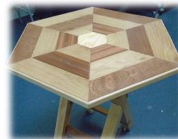
**Bruno** made his table from pine and laser-etched some inspirational messages across the top. The joints he hand-cut were of a really good standard and included both cross halving and dovetail joints. The top is made from laminated solid pine and has a routed rounded edge. Each part of the table was made with care and a high level of accuracy.
